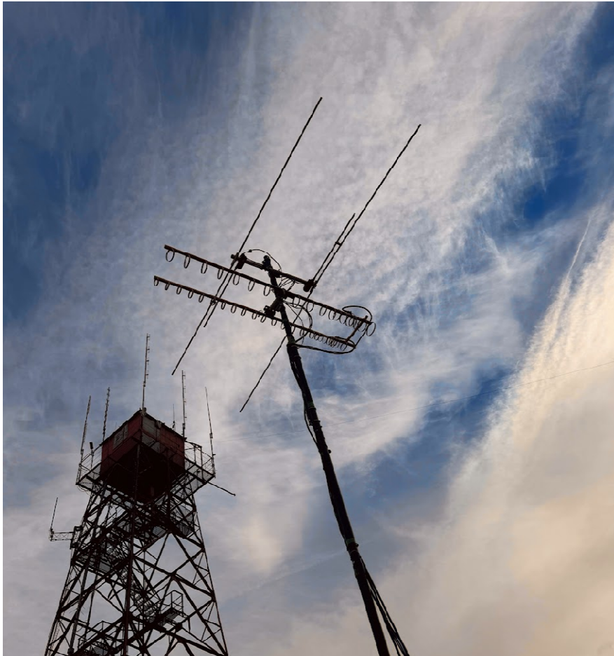
Antenna test at the Ebright Azimuth in Delaware with Looper antennas mounted on a quick mount
